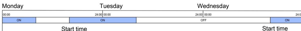
Figure 16: If an ON-time runs past midnight on a day when the 24-hour clock is not active, the function will remain ON until the time has elapsed.
